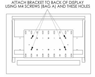
Figure 6. Display with 300mm x 100mm Hole Pattern
